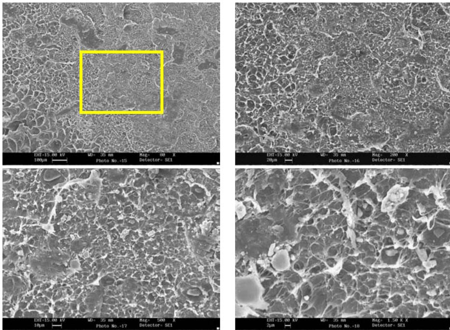
Figure 4: SEM Images from Fracture Surface at Inner Liner Location on Field Pipe
