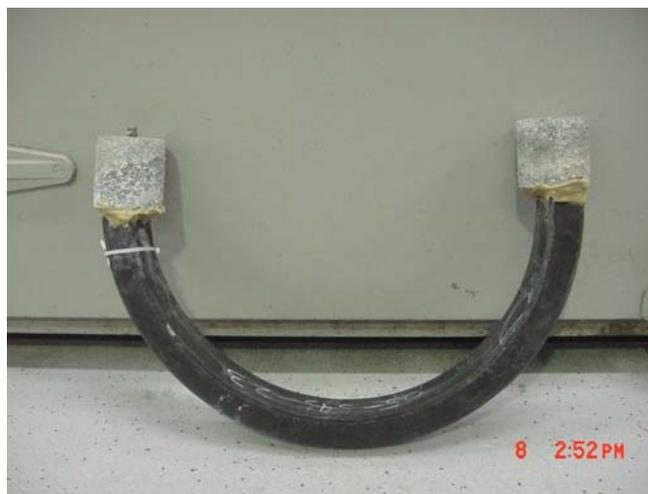
Figure 1: Pipe Ring Test Specimen
