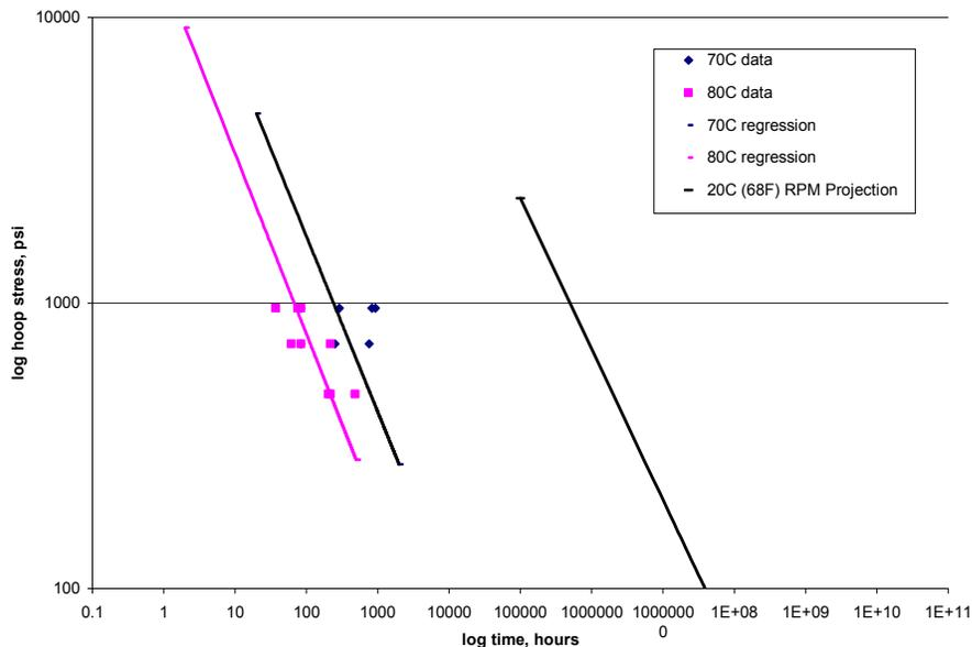
Figure 6: RPM Analysis of Recycled HDPE Corrugated Pipe
