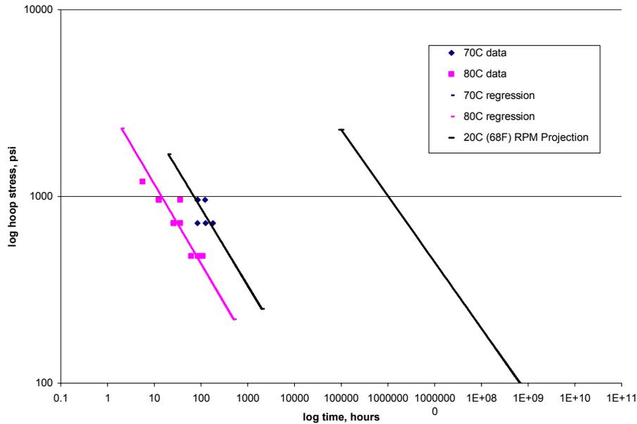
Figure 5: RPM Analysis of Control HDPE Corrugated Pipe
