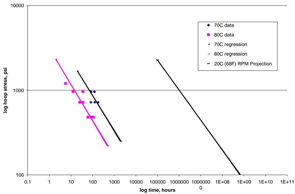
Figure 6: RPM Analysis of Control Corrugated HDPE Pipe
