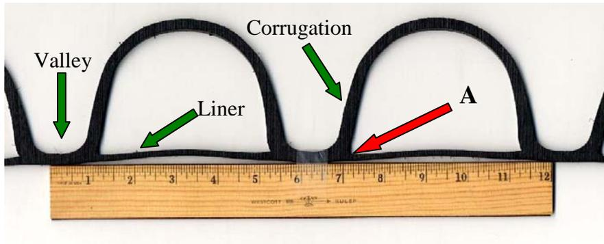
Figure 5 – Corrugation HDPE Pipe Profile
