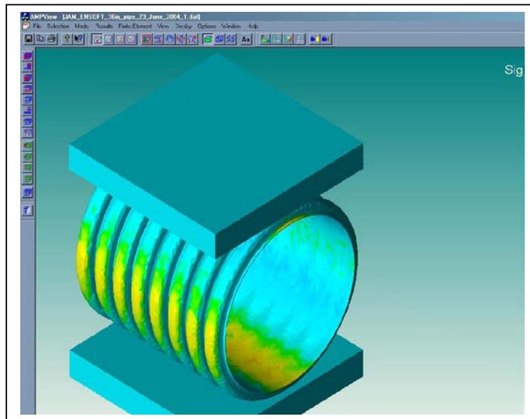
Figure 2 – High Stress Locations Associated with Parallel Plate Loading
