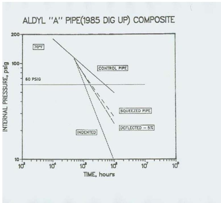
Figure 4 – Composite Showing Control Pipe and Secondary Loading Effects
